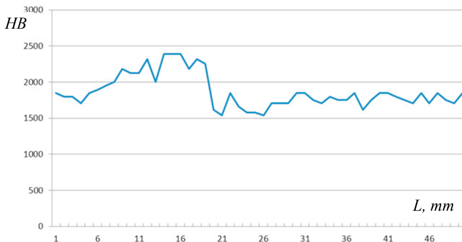
Fig. 2. HB microhardness distribution for HAZ of St3sp weld steel probe after low-cyclic fatigue test.
